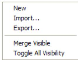
You can use this to create a new relief layer, import triangle and surface models onto a relief layer, export a relief, duplicate a relief layer, move a relief layer to the opposite stack, merge relief layers, create a greyscale bitmap layer, delete a relief layer, and toggle the visibility of relief layers in the stack associated with the model's back surface.
