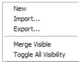
You can use this to create a new relief layer, import triangle models, surface models or relief clipart, and toggle the visibility of relief layers.
