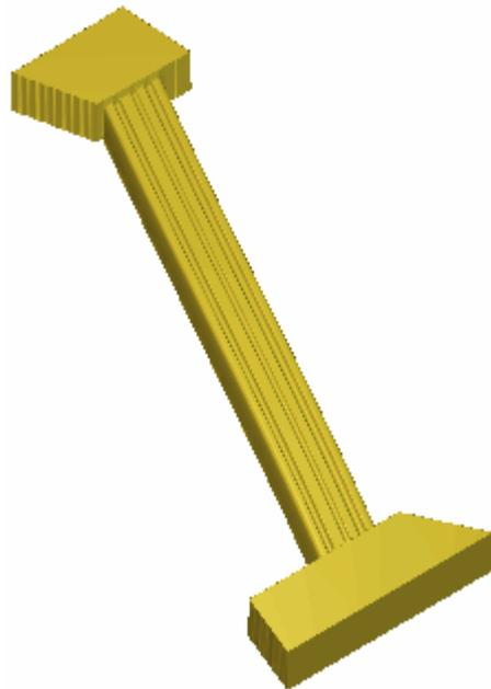
Prior to calculating the extruded shape, the blocks at the top and bottom of the harp frame were created by applying a flat profile with a shallow height to the red bitmap colour using the **Shape Editor**.
